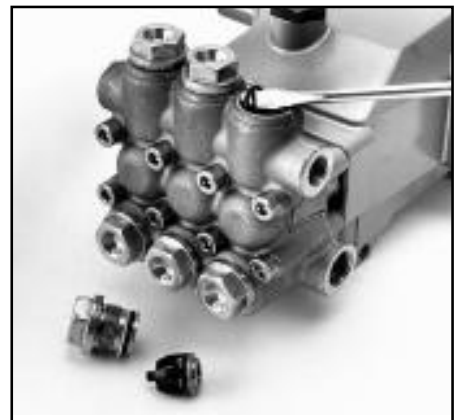
All Models Removal of Valve Seat O-Ring
